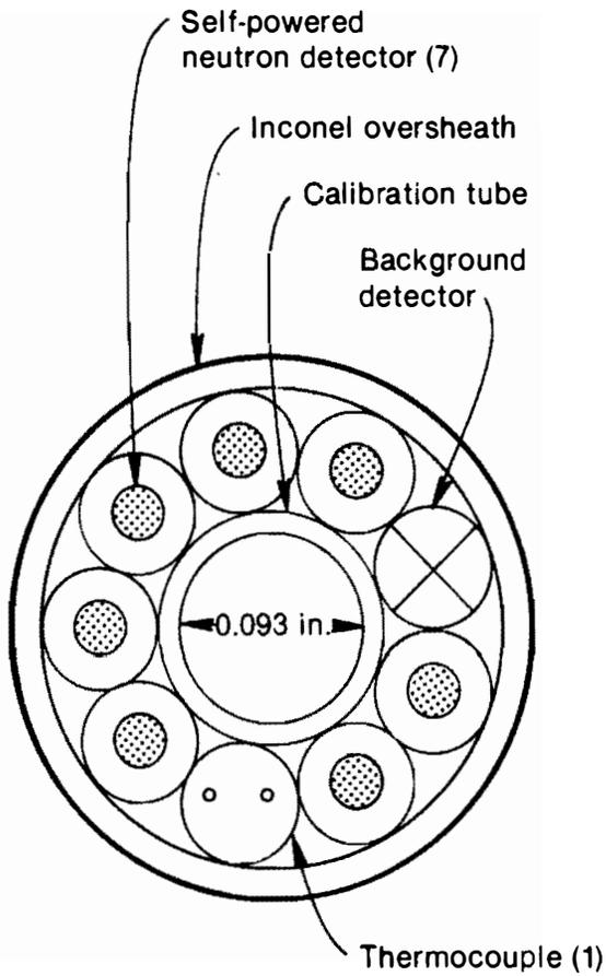
a. Fixed SPND assembly cross section
