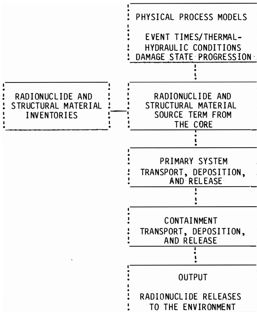
Figure 1. Key steps involved in analyzing the release and transport of radionuclides in light water reactors.
