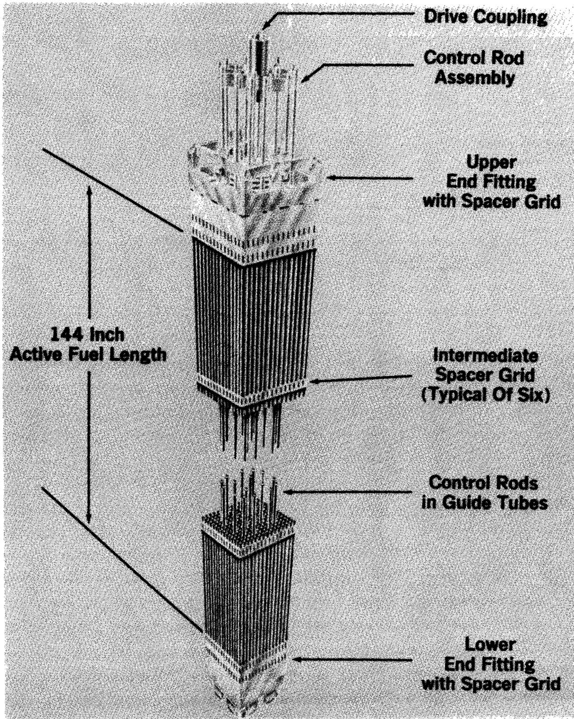
Figure 10. Typical TMI-2 fuel assembly.
