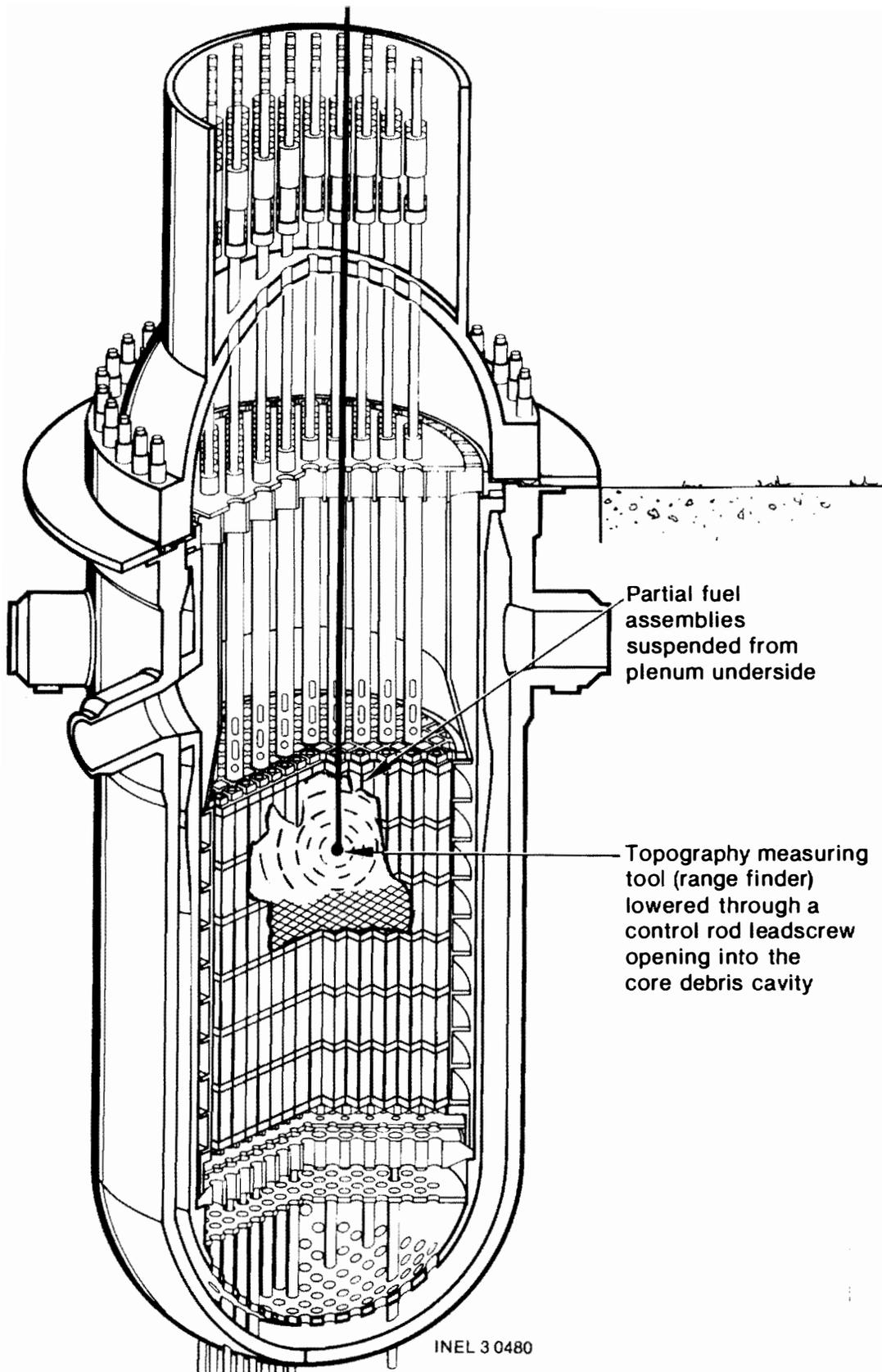
Figure 13. Schematic showing topographic measurement of core damage features.
