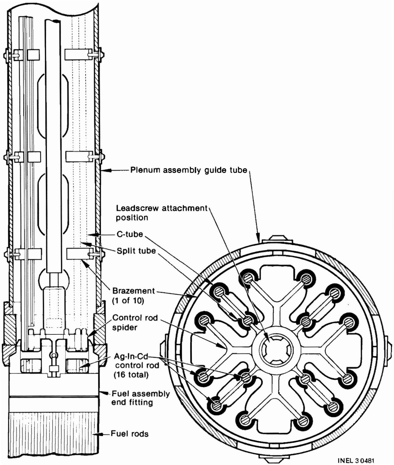
Figure 8. Vertical and horizontal cross section of plenum guide tube assembly.
