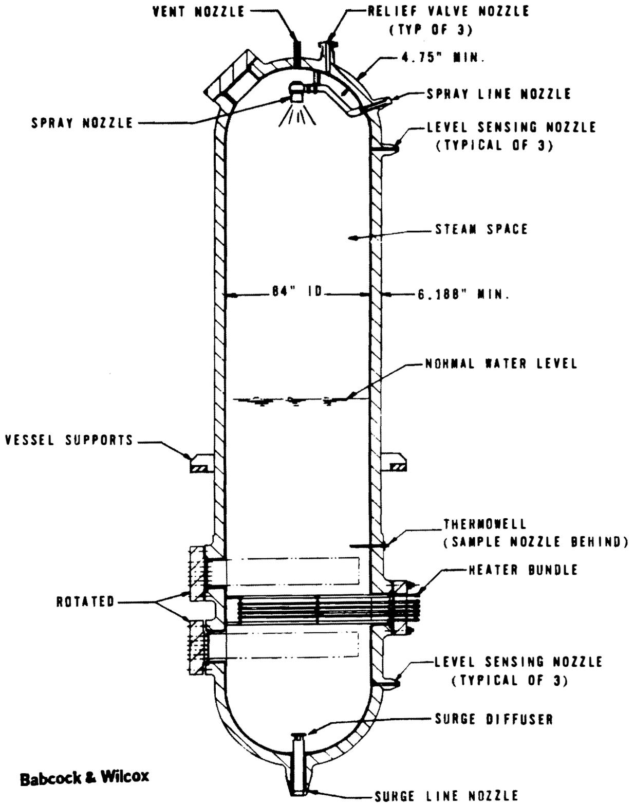
Figure 17. TMI-2 pressurizer vessel and internals.
