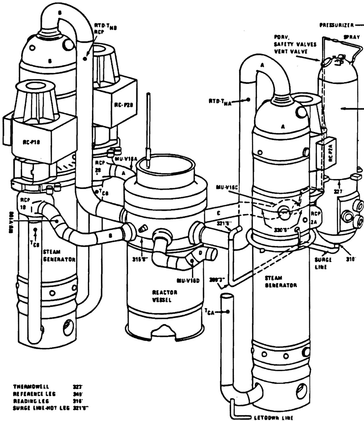
Figure 15. Schematic of the TMI-2 reactor coolant system.
