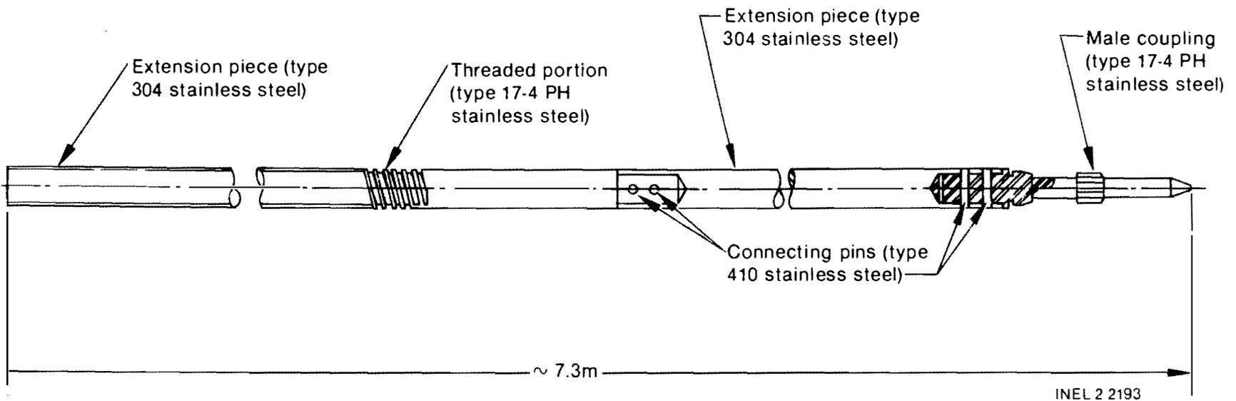
Figure 2. Schematic of a control rod drive leadscrew.
