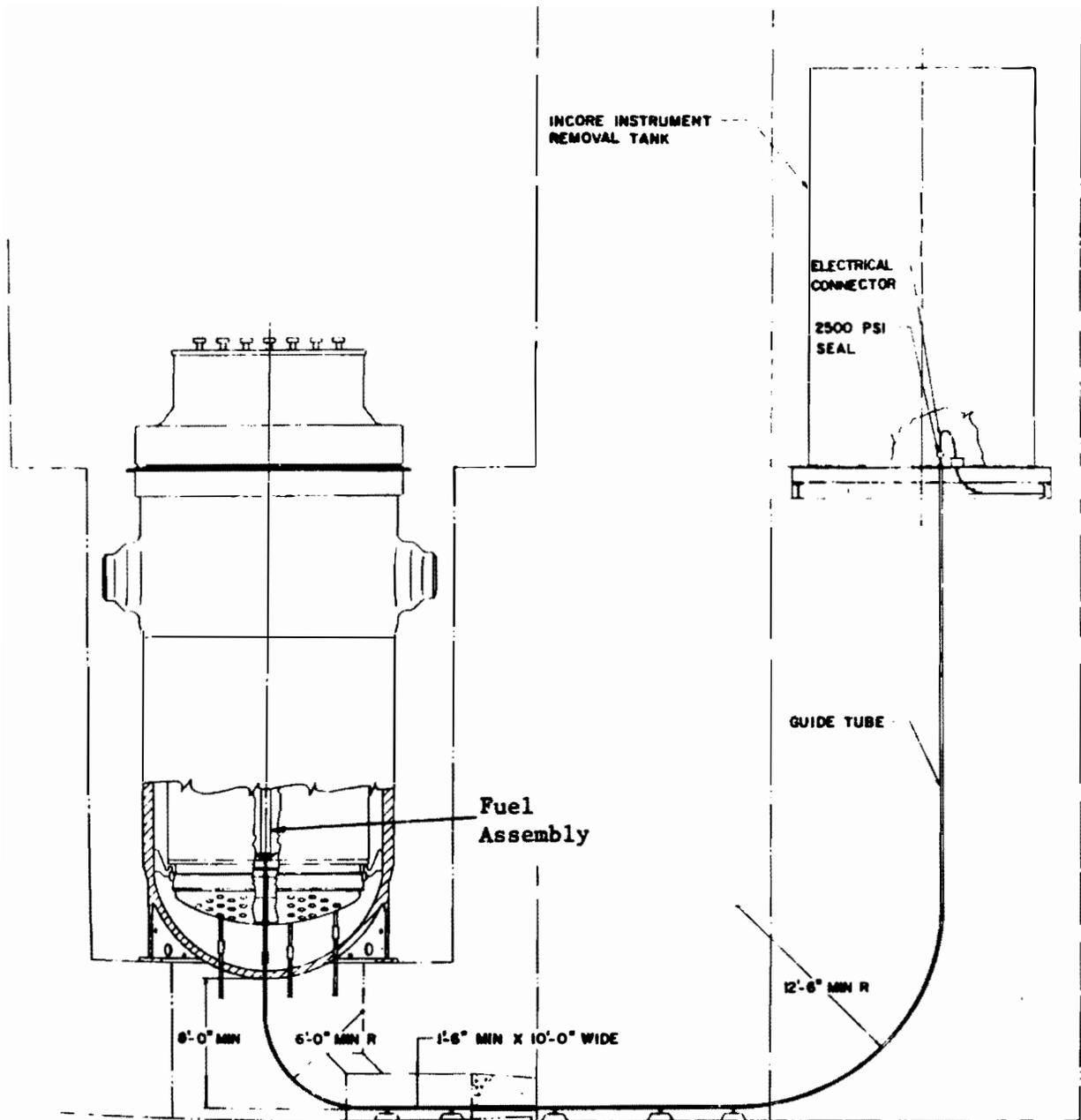
Figure 14. Schematic of a typical instrument detector assembly installation.
