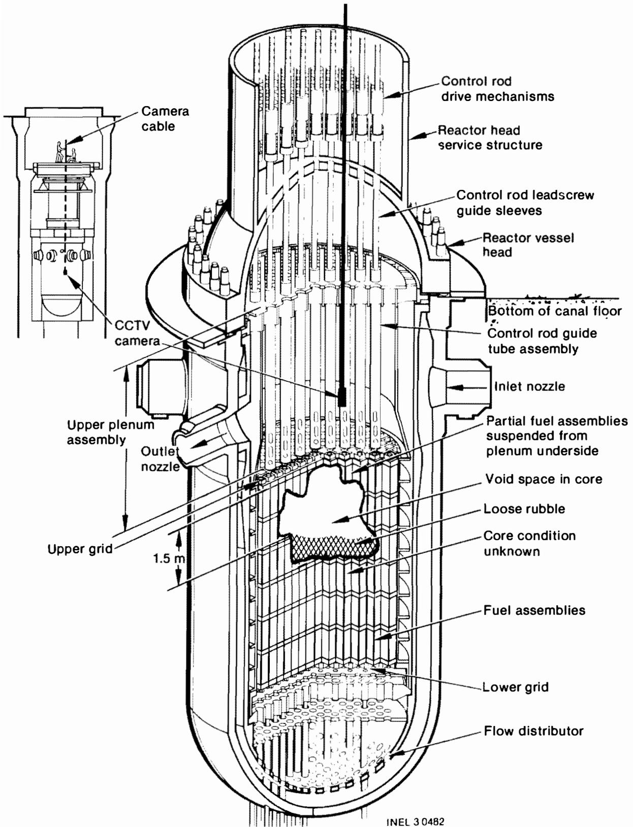
Figure 11. Closed-circuit television camera being lowered into the TMI-2 reactor.
