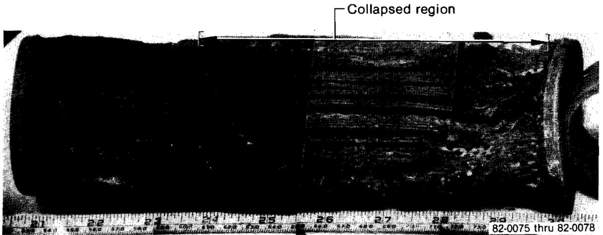
(b) Filter MUF-4A (collapsed as a result of differential pressure)
