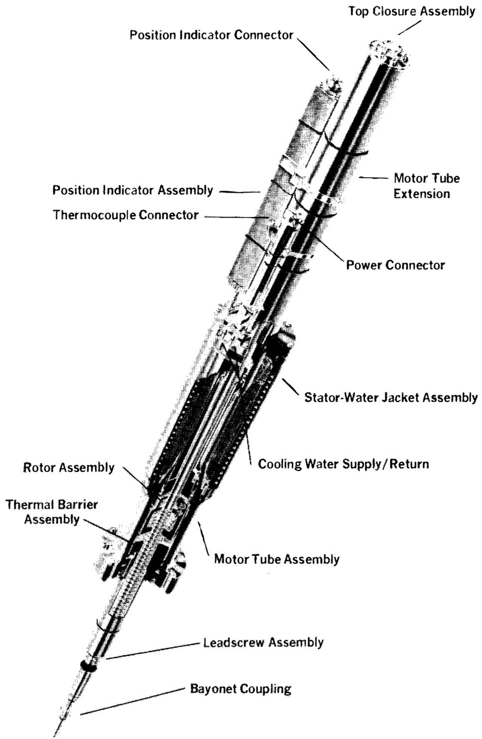
Figure 3. Typical TMI-2 control rod drive mechanism.
